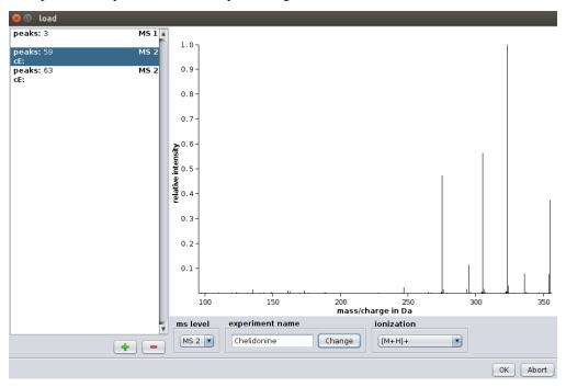
For each spectrum you have to select the MS level (either MS1 or MS/MS). If you have MSn spectra you can just import them as MS/MS spectra. You can select a name for the compound as well as an ionization mode. The collision energy is an optional attribute as it does not affect the computation.
