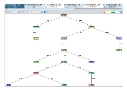
The *Tree view* tab displays the estimated fragmentation tree. Each node in this tree assigns a molecular formula to a peak in the (merged) MS/MS spectrum. Each edge is a hypothetical fragmentation reaction. The user has the choice between different node styles and color schemes.
