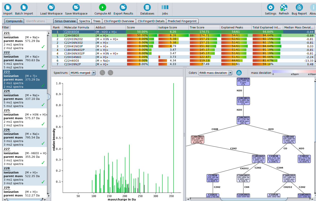
Fig. 3. Additional candidates are added to the SIRIUS Overview tab after searching with CSI:FingerID in a structure database considering adduct types [M + H]^+ , [M + NH_4]^+ and [M - H_2O + H]^+ . Molecular formulas C_{24}H_{40}O_4 and C_{24}H_{38}O_3 differ by an in-source loss of H_2O and are not distinguishable by MS/MS since in both cases, the ion [C_{24}H_{38}O_3 + H]^+ is fragmented; hence, both have identical score. (The same holds for the pairs C_{22}H_{33}N_2O_2 vs. C_{22}H_{36}N_3O_2 and C_{18}H_{39}N_4O_2P vs. C_{18}H_{36}N_3O_2P .) Displayed is the resolved fragmentation tree for [C_{24}H_{40}O_4 - H_2O + H]^+ , where an H_2O loss has been added to its top.
