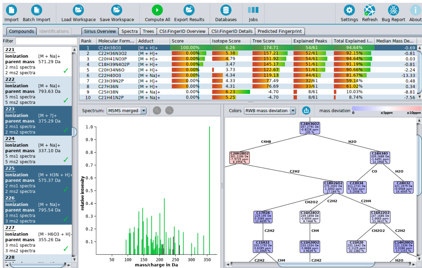
Fig. 1. The SIRIUS Overview tab displays the spectrum and fragmentation trees of the top molecular formula candidates. The best candidate C 24 H 38 O 3 is selected; the corresponding explained spectrum and fragmentation tree are shown. The left panel contains a searchable list of all compounds; selected compounds are highlighted. The data and results of the first selected compound are displayed in all the views to the right of the compound list. The upper panel provides functionalities to import spectra, save and load workspaces, export result tables, start computations and display their status in the jobs panel. The SIRIUS overview tab displays various scores for each molecular formula candidate and can be sorted accordingly.
